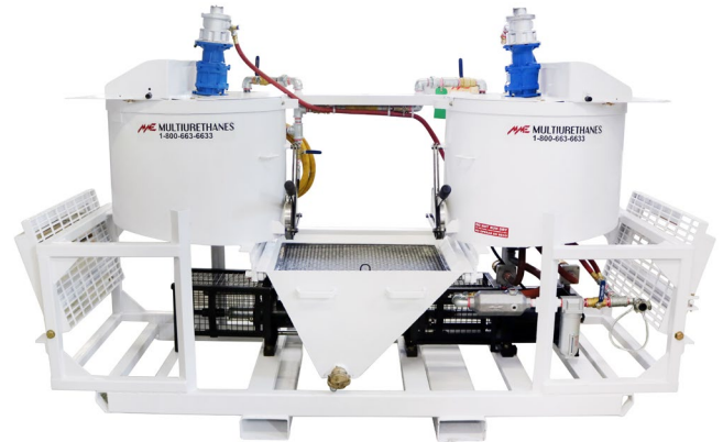
Front view of the CG-500-3X8/A with safety upgrades and optional components.
